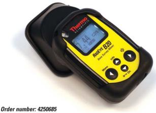
The RadEve B20 is a modern compact multi-purpose contamination meter for alpha, beta, gamma and X-ray radiation. By virtue of an optional gamma energy filter, gamma dose rate measurements from 17 – 1300 keV can be performed. For emergency response purposes alpha and beta contamination can be discriminated using another optional filter.
