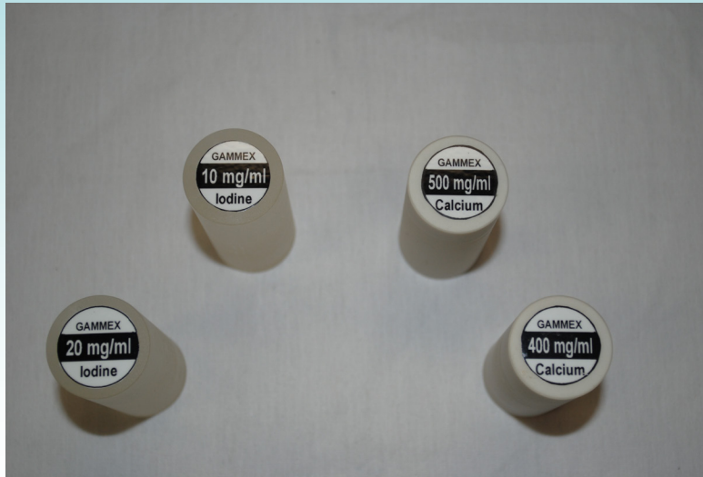
Calcium and Iodine rods of various concentrations permit easy analysis of detection ranges.
